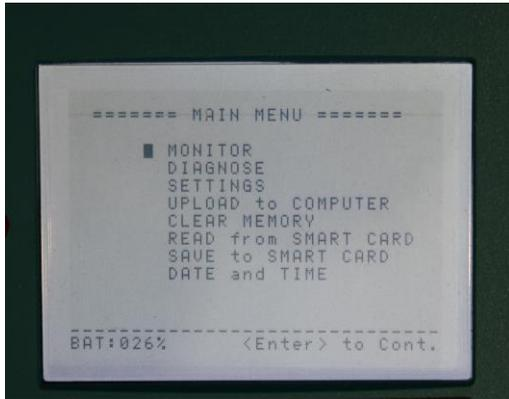
Within one second BAMbino will be scanning its acoustic environment, listening for noises characteristic of bearing faults **with the settings of the Active** Location.
