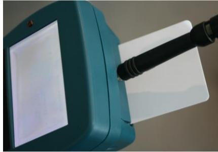
You can save your settings to the smart card by inserting the smartcard as shown above, then selecting *SAVE to SMART CARD* from the menu.
