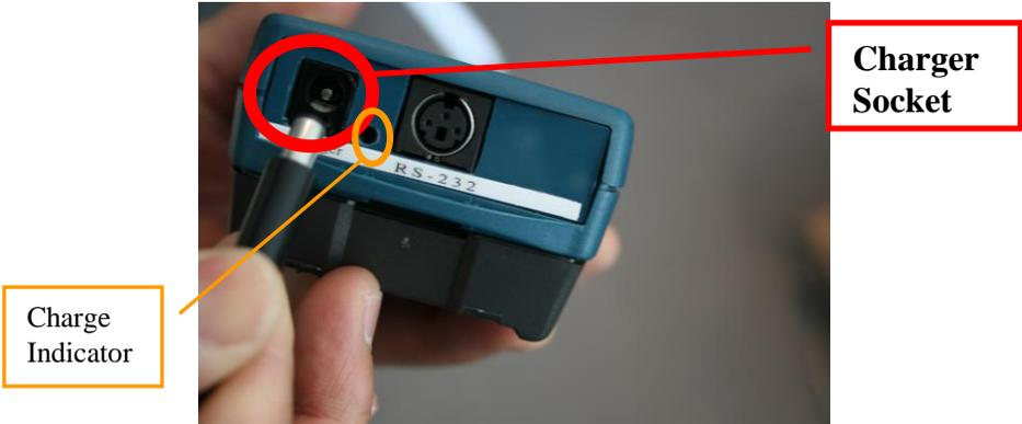
The Charge indicator lamp will remain on while the unit is charging and turn off when the charge is complete.
