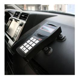
A compact, brake performance tester that uses a multi-channel sensor to measure tri-axial deceleration of any type of vehicle or motorcycle, making it one of the most versatile brake testers on the market.
