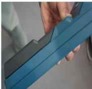
plug the power pack into a 240V wall socket and into the BAMbino. The BAMbino will need a 4 hour charge to completely charge the batteries, the charge cycle will automatically stop when the charge is complete
