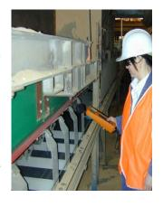
is a "quick look" mode of operation that is used for quickly indicating the presence of a faulty bearing. When the instrument detects a noise that is characteristic of a faulty roller, an alarm is set off and the operator would then stop and mark the roller. There is a note pad facility to allow the user to write a comment, and the operator also has the ability to enter the diagnosis mode to display an instantaneous frequency spectrum of the faulty bearing.
