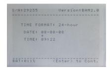
The Date should be entered using the number keys until the correct date is entered, after each digit is entered the cursor will advance to the next digit. If an incorrect digit is entered then you can go back a space by selecting the shift mode and pressing
