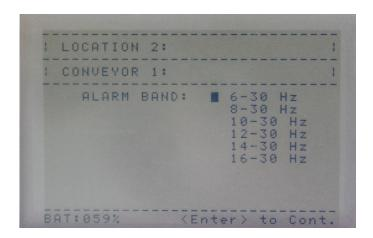
Scroll through the Alarm Bands using the arrow buttons.
