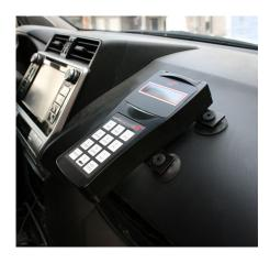
A compact, brake performance tester that uses a multi-channel sensor to measure tri-axial deceleration of any type of vehicle or motorcycle, making it one of the most versatile brake testers on the market.
