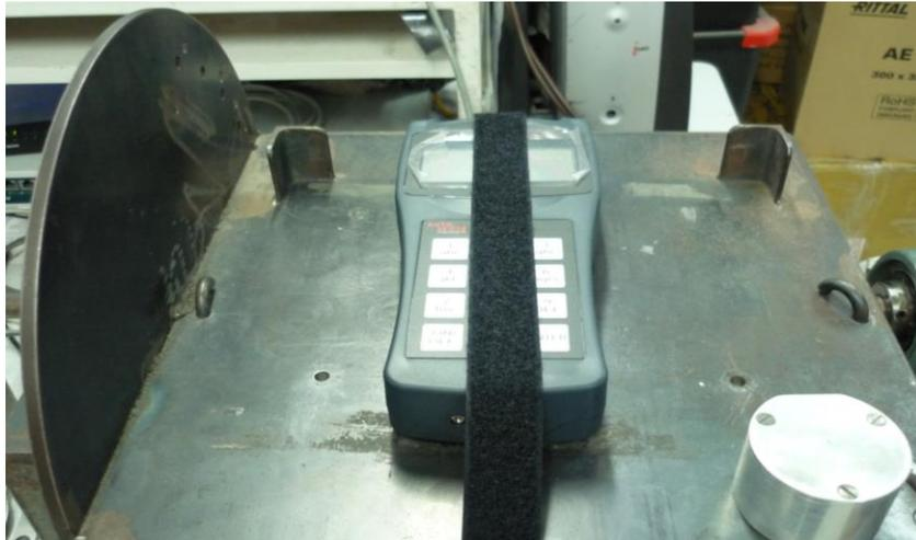
*Figure 66. Suspension Meter – X Axis*
