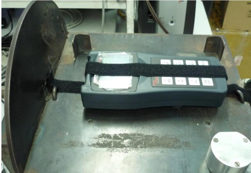
Figure 72. Suspension Meter Calibration – Y Axis
