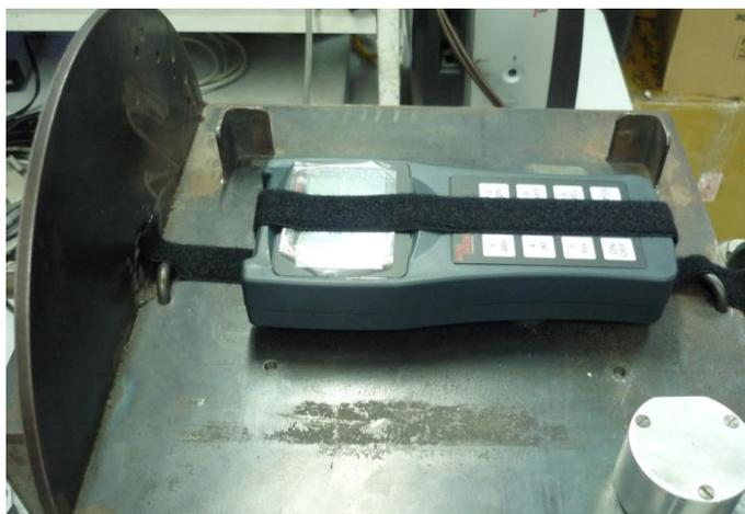
Figure 75. Suspension Meter Calibration – Y Axis position 3
