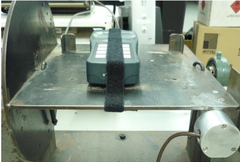
*Figure 78. Suspension Meter Calibration – Z Axis*
