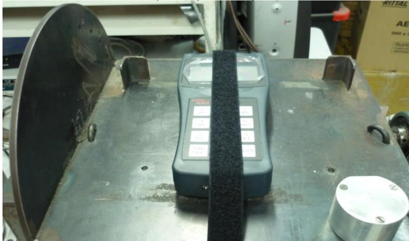
Figure 69. Suspension Meter Calibration – X Axis position 3
