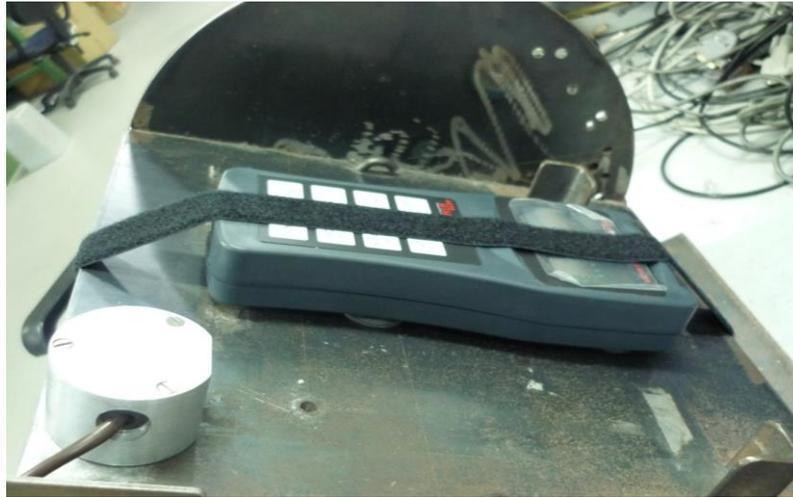
Figure 68. Suspension Meter Calibration – X Axis position 2
