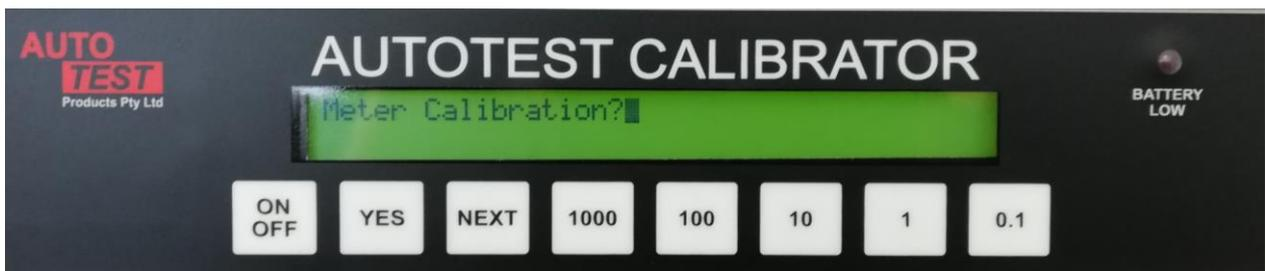
Figure 1. The Front Panel of the Auto Test Calibrator
