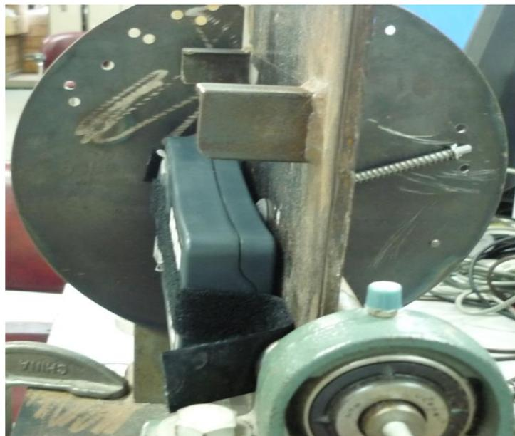
Figure 77. Suspension Meter Calibration – Y Axis position 5
