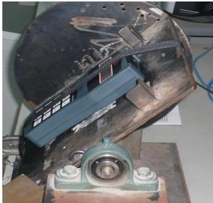
Figure 43. MiniPlus Calibration – Z Axis position 1
